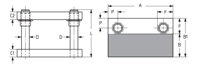
When the overall size of die set has been determined, our recommendations for minimum plate thickness and suggested diameters of guiding elements are indicated in the table below. **Note:** These can be varied to suit customer requirements.
